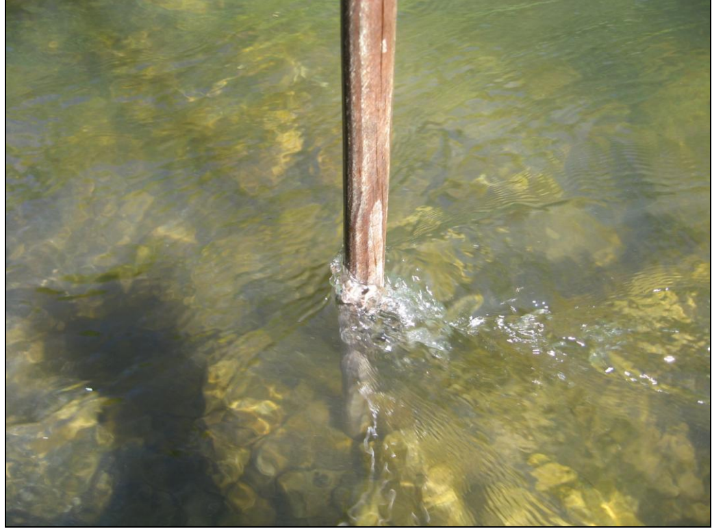
Figure 4-7: Critical Flow Wave Action on Wading Staff
