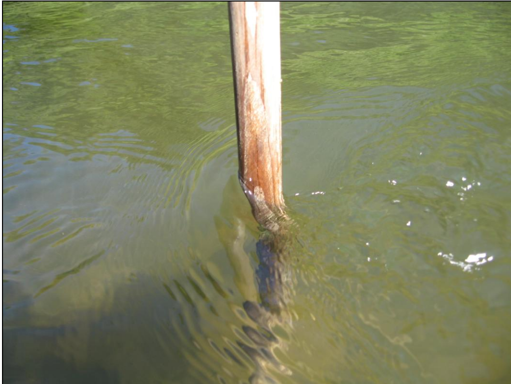
Figure 4-6: Sub-Critical Flow Wave Action on the Upstream Side of a Wading Staff
